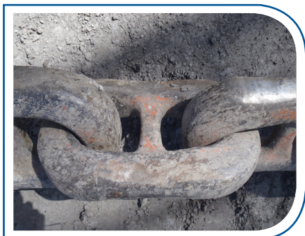
3" Dump Chain after 2million BCM's
