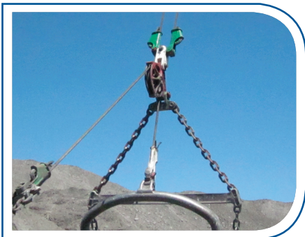
Previous Upper Hoist Rigging Setup
